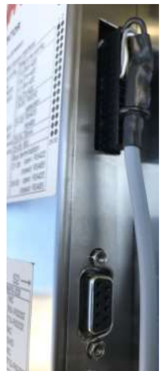
serial S2 9 pol. DSUB socket RS232
