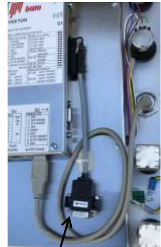
Adapter to S1 Art.-no. 801141 9 pol. DSUB plug 20 mA
