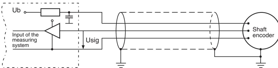
In case of absolutely parallel measuring systems, the number of the signals to be measured depends on the resolution of the encoder. For these encoders, the operating and signal voltage is within a range of 15 - 24V. The maximum amplitude of the noise voltage must not exceed the value of 3.5V.
